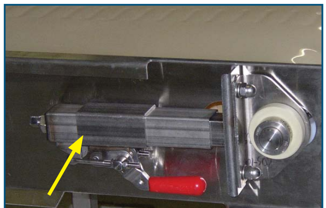
Figure 6: Example of quick release take-up mechanism
