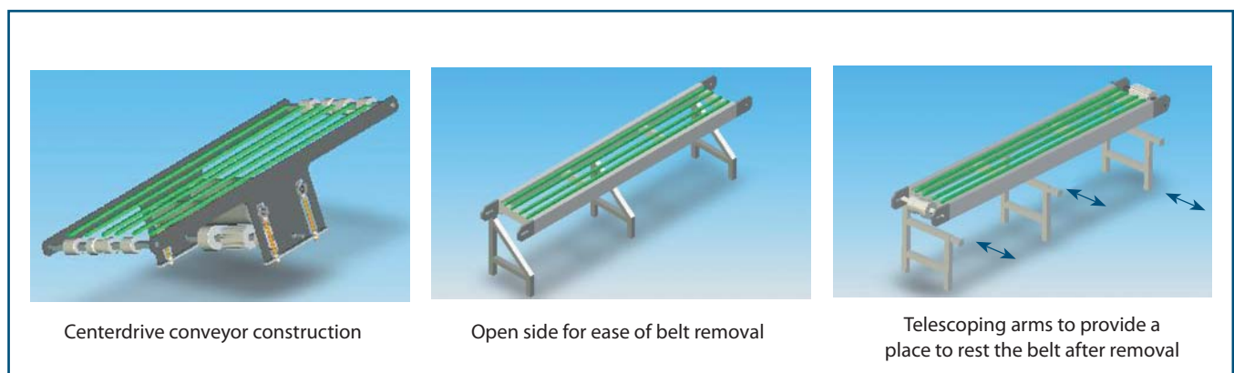
Figure 8: Optional conveyor constructions
