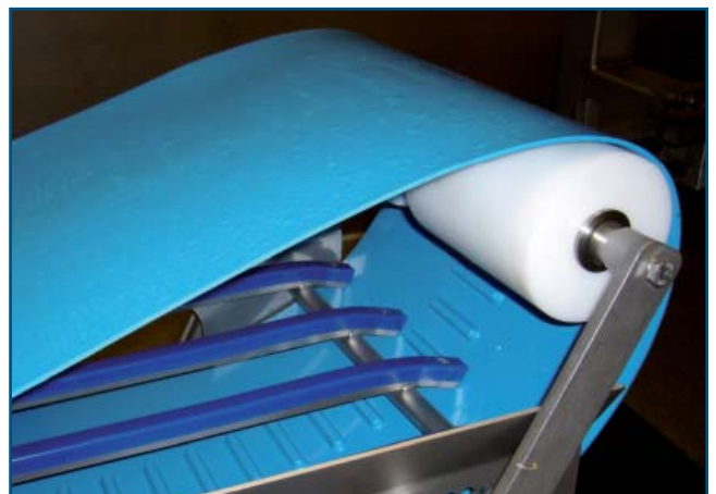
FHB-3-SD: Shows the tail pulley and slidebed
