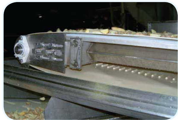
FHW-3-SD Integral teeth function as a guide for the belt
