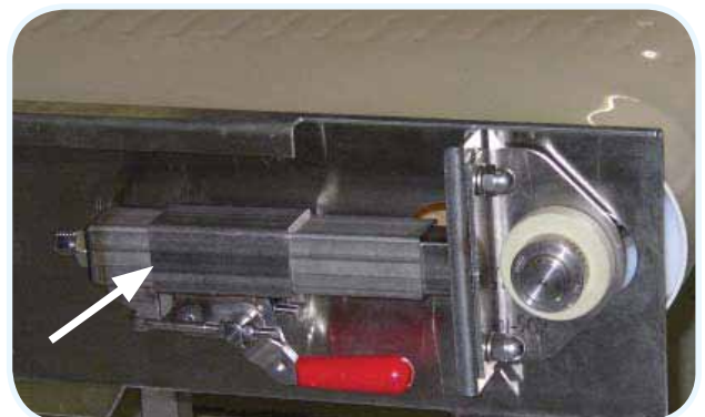
Example of Quick Release Tensioner Mechanism
